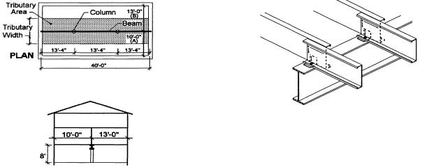
Solution: One continuous beam with two columns equally spaced is chosen. The top flange of the beam is to be braced at each joist (a positive connection is necessary between each joist and the beam). Provide a minimum of  $1\frac{3}{4}$  inches of bearing at the beam ends and  $3\frac{1}{2}$  inches of bearing at each column.
