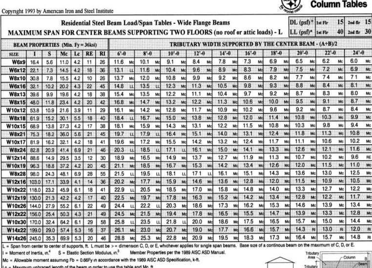
Lc = Maximum unbraced length of the beam in order to use this table and Mc, ft.
