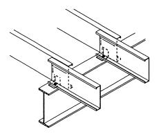
Solution: One continuous beam with two columns equally spaced is chosen. The top flange of the beam is to be braced at each joist (a positive connection is necessary between each joist and the beam). Provide a minimum of 13 inches of bearing at the beam ends and 3½ inches of bearing at each column.
