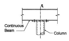
Simple beam loads = 13.33[11.5(10+10+40+30) + 39 + 15]= 14,516 lbs. Simple beam end reaction = (14,516)/2 = 7,258 lbs.
